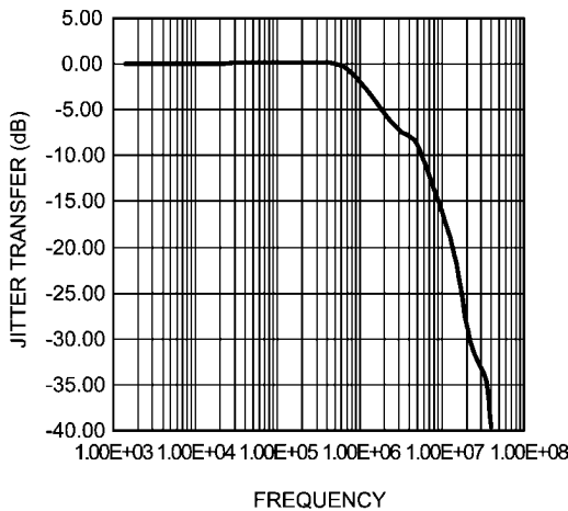
FIGURE 8. Jitter Transfer Curve
